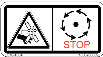
Fig. 22: Fan in engine compartment
