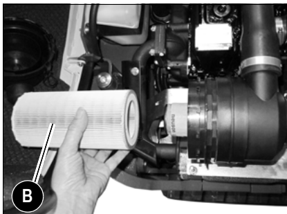
Fig. 152: Removing the outside air filter
