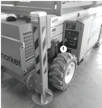
Figure 6.1.1 - Control Box Location, Ground Position
