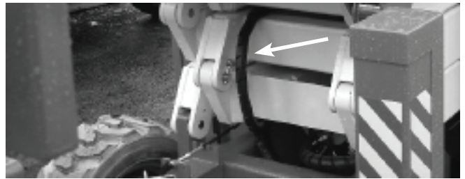
Figure 7.11 - Wiring Harness in the Scissor Stack
