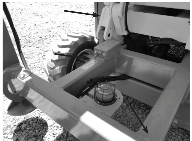
Figure 7.19 - Structural Damage and Welds
