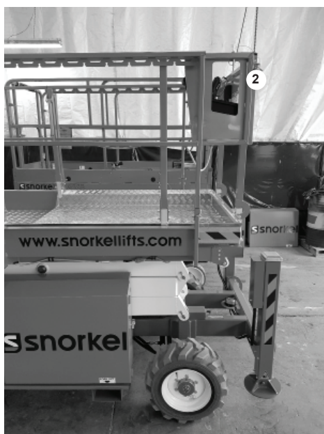
Figure 6.1.2 Control Box Location, Platform Position
