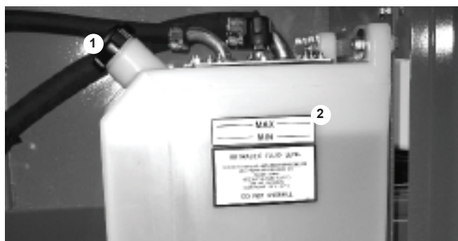
Figure 7.13 - Hydraulic Oil Tank
