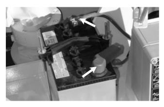
Figure 7.7 - Battery Terminals
