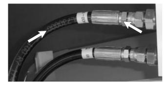
Figure 7.12 - Hydraulic Oil Leaks At Fittings And Hoses
