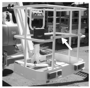
Figure 2.4 - Gravity Gate
