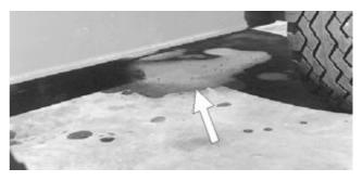
Figure 7.11 - Hydraulic Oil Leaks
