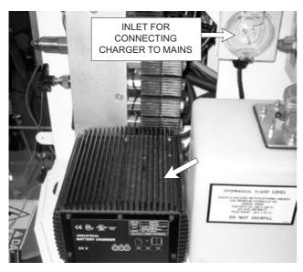
Figure 11.6 - On-Board Battery Charger
