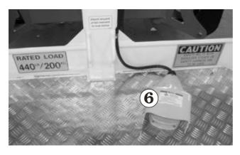
Figure 8.11 - Platform Foot Switch
