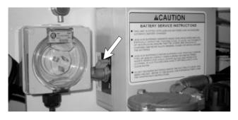
Figure 11.2 - Master Battery Isolate Switch
