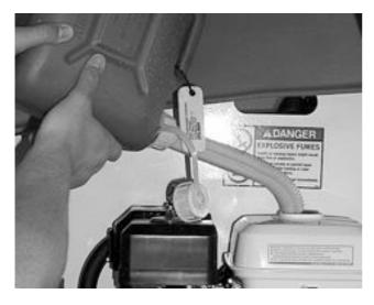
Correct Method to Fill MHP13/35 / MHP15/44 Mark II Fuel Tank
