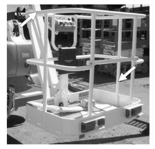
Figure 2.5 - Guardrails
