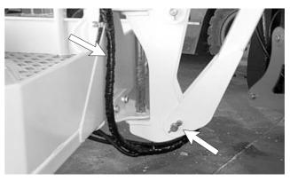
Figure 7.6 - Wiring Harnesses
