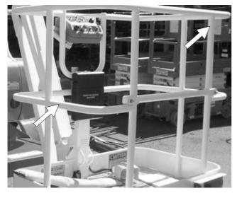
Figure 7.20 - Platform Guardrails
