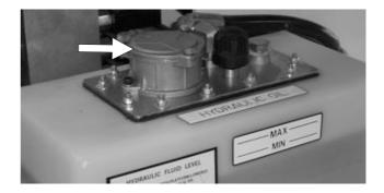
Figure 7.10 - Hydraulic Oil Filler Cap
