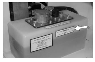
Figure 4.3 - Hydraulic Oil Level
