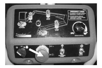
Figure 8.2 - Platform Control Box Emergency Stop Switch Location.
