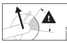
Kickback occurs when the cut-off machine is suddenly thrown up and back in an uncontrolled arc towards the operator.
