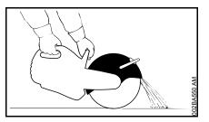
Set the abrasive cutting wheel guard correctly: Guide particles of material away from the user and machine.
