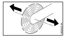
When a cut-off machine with an abrasive cutting wheel rotating is moved in the direction of the arrow, a force is produced which causes the machine to tip sideways.
