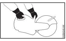
Always hold the machine **firmly with both hands**: Right hand on the rear handle – even if you are left-handed. To ensure safe control, wrap your fingers tightly around both handles.
