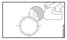
• First lateral cut on the top half of the pipe
