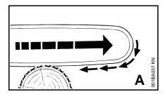
Pull-in occurs when the chain on the bottom of the bar is suddenly pinched, caught or encounters a foreign object in the wood. The reaction of the chain pulls the saw forward.
