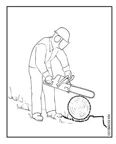
If on a slope, stand on the uphill side of the log. Watch out for rolling logs.
