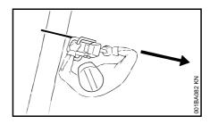
Position the saw so that your body is clear of the cutting attachment.
