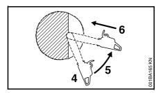
Begin cut (4) by applying lower portion of the guide bar nose – do not use upper portion because of risk of kickback. Cut until depth of kerf is twice the width of the quide bar.
