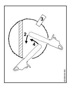
When repositioning for the **next cut (2)**, keep the guide bar fully engaged in the kerf to keep the felling cut straight – apply the spiked bumper again.
