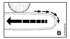
Pushback occurs when the chain on the top of the bar is suddenly pinched, caught or encounters a foreign object in the wood. The reaction of the chain drives the saw straight back toward the operator.
