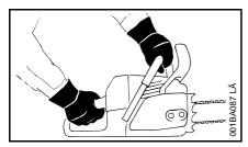
Always hold your saw firmly with both hands – right hand on the rear handle, even if you are left-handed. To ensure safe control, wrap your fingers tightly around the front handle and control handle.
