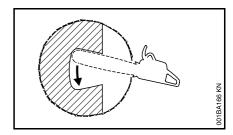
Carefully make the plunge cut in the center of the felling notch – there is a danger of pushback at this point – then swing the bar in the direction of the arrow.
