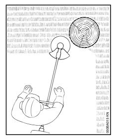
Nylon line achieves soft cut for edging and trimming around trees and fence posts – less risk of damaging tree bark.
