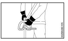
Versions with loop handle and loop handle with barrier bar: Left hand on loop handle, right hand on control handle on drive tube.
