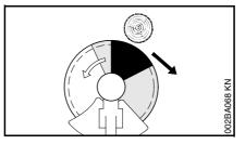
The risk of kickout is highest in the **black area** area of the blade: Do not use this area of the circular saw blade for cutting.
