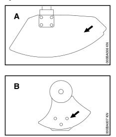
The **direction of rotation** of the cutting tool is indicated by an **arrow** on the deflector (**A**) for all mowing tools and the stop (**B**) for circular saw blades.
